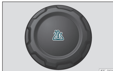
Fig. 205 Engine compartment: coolant expansion tank cap.
