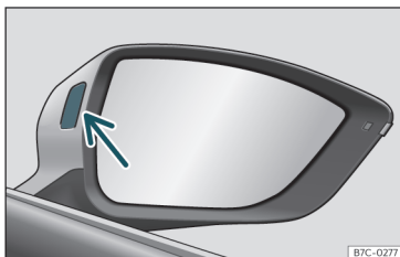
Fig. 171 Control lamp of the lane departure warning.
