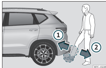
Fig. 85 Rear lid with sensor-controlled opening (Easy Open).
