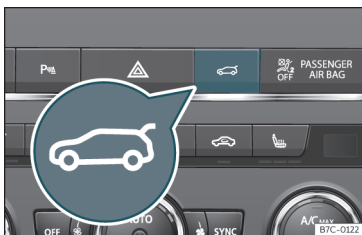
Fig. 84 Centre console: button to open and close the rear lid.
