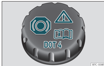
Fig. 206 Engine compartment: brake fluid reservoir cap.
