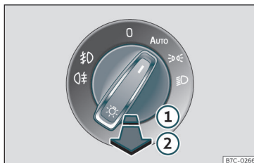
Fig. 93 Dash panel: lights control.
