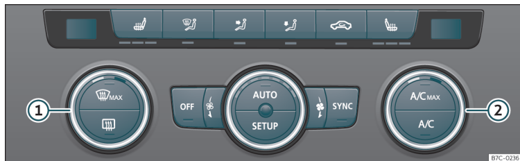
Fig. 129 In the centre console: Climatronic controls.
