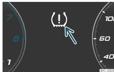
Fig. 212 Instrument panel: warning of loss of tyre pressure.
