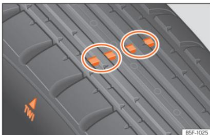
Fig. 230 Tyre profile: tread wear indicators.
