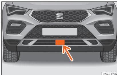
**Fig. 167** On the front bumper: radar sensors.
