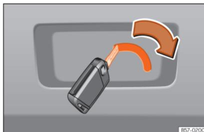
**Fig. 102** Detail of the luggage compartment: emergency unlocking
