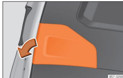
**Fig. 61** Rear lid open: remove the cover.
