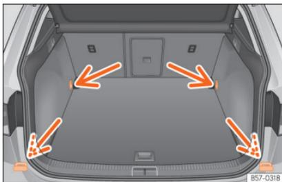
**Fig. 132** In the luggage compartment: fastening rings.
