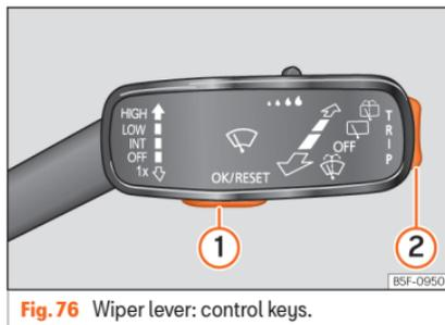
Fig. 76 Wiper lever: control keys.
