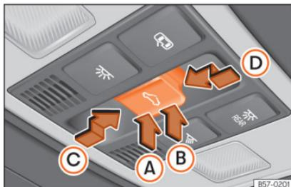
**Fig. 104** On the interior roof lining: sunroof button.
