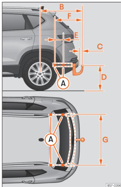
**Fig. 215** Limits and attachment points for retrofitting a towing bracket.
