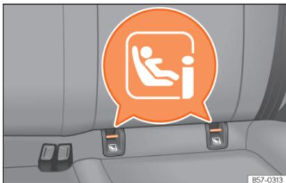
**Fig. 26** Rear seat: ISOFIX/i-Size securing rings.
