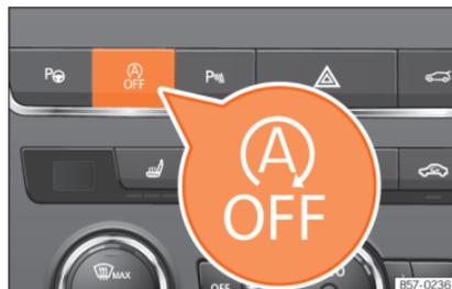
**Fig. 160** Centre console: Start-stop system button.
