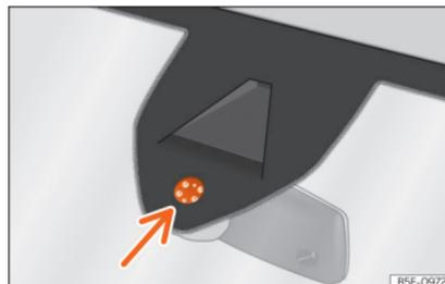
**Fig. 114** Rain sensor sensitive surface
