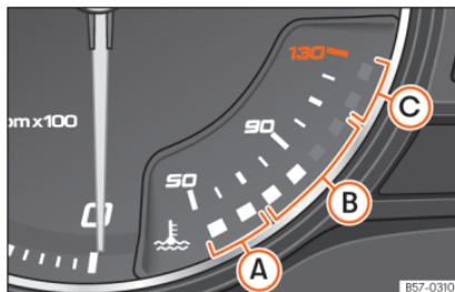
**Fig. 73** Analogue instrument panel: engine coolant temperature indicator.
