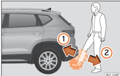
**Fig. 100** Rear lid with sensor-controlled opening [Easy Open].
