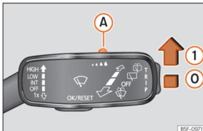
**Fig. 113** Wiper lever: adjust the rain sensor **A**
