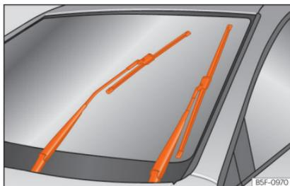
Fig. 40 Wipers in service position.
