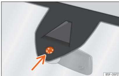
**Fig. 147** Windscreen humidity and temperature sensor.
