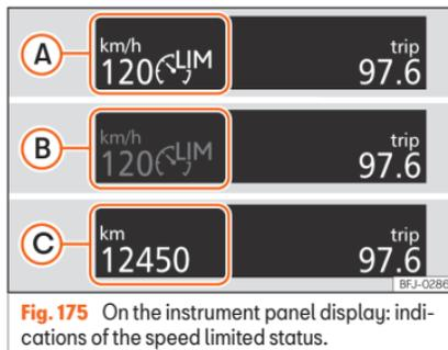
**Fig. 175** On the instrument panel display: indications of the speed limited status.
