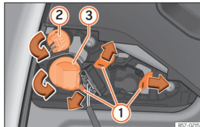
**Fig. 62** Remove the bulb holder.
