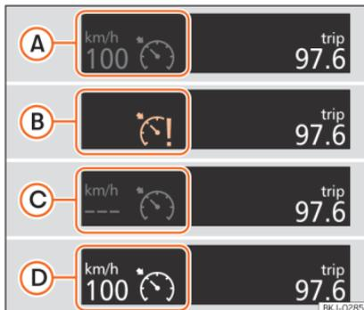
**Fig. 173** Instrument panel display: GRA status indications.
