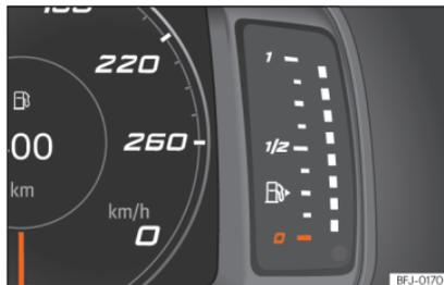
**Fig. 72** Digital instrument panel: fuel gauge.
