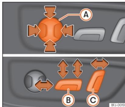
Fig. 118 Driver's seat: electric seat settings.
