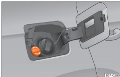
**Fig. 218** AdBlue tank cap.**Operations prior to refilling**
