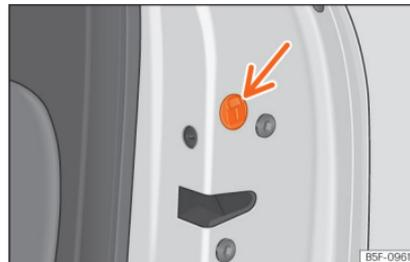
**Fig. 95** Locking the door manually.
