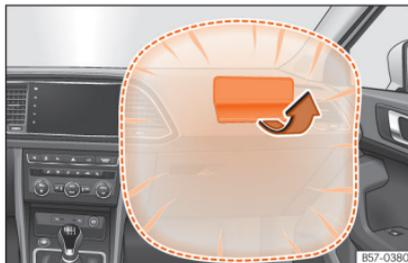
**Fig. 15** Front passenger airbag located in dash panel.
