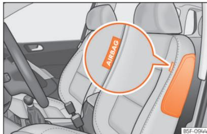
**Fig. 20** Side airbag in driver's seat.
