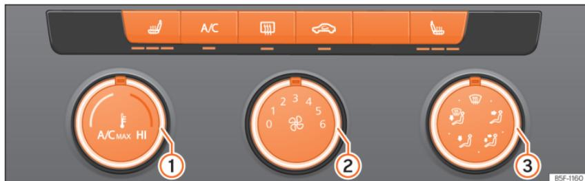
**Fig. 146** In the centre console: Manual air conditioning controls.
