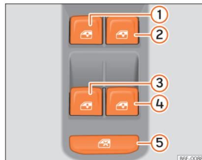
**Fig. 103** Detail of the driver's door: window controls.
