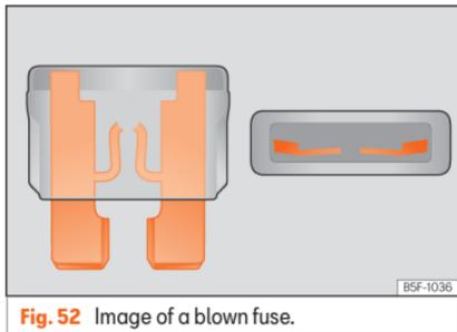
**Fig. 52** Image of a blown fuse.
