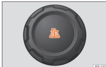
**Fig. 225** Engine compartment: coolant expansion tank cap.
