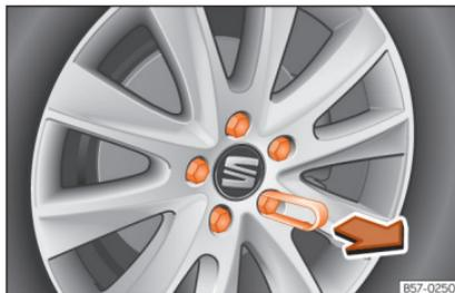
**Fig. 34** Wheel: wheel nuts with caps.
