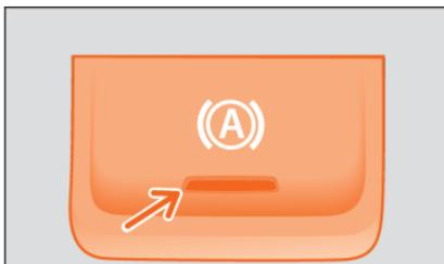
**Fig. 195** In the lower part of the centre console: Auto Hold function button.
