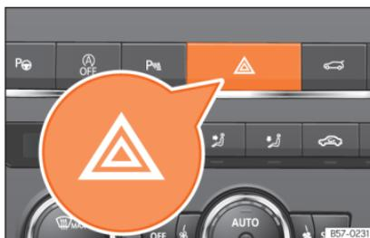
**Fig. 110** Dash panel: hazard warning lights switch
