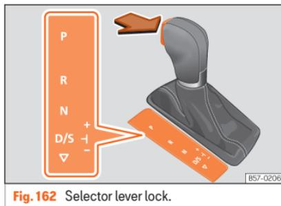
Fig. 162 Selector lever lock.
