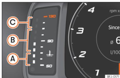
**Fig. 74** Digital instrument panel: engine coolant temperature indicator.
