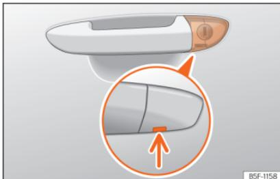
**Fig. 93** Driver door handle: Concealed lock cylinder.
