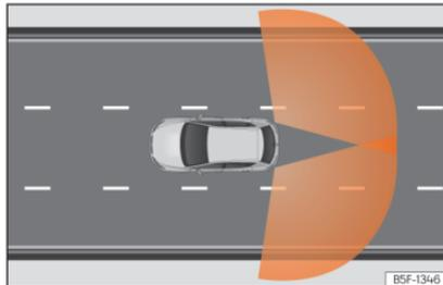
**Fig. 171** Sensor detection zones
