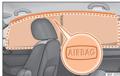
**Fig. 22** Location of head-protection airbags.
