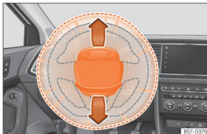
**Fig. 14** Driver airbag located in steering wheel.
