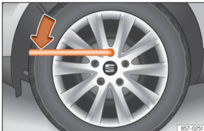
**Fig. 36** Wheel change: loosen the wheel nuts.
