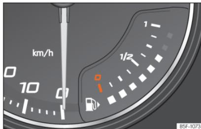
**Fig. 71** Analogue instrument panel: fuel gauge
