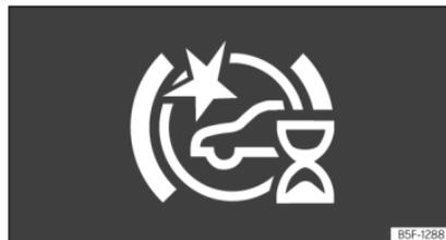
**Fig. 177** On the instrument panel display: initial system self-calibration indication.
