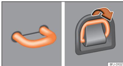
**Fig. 131** In the luggage compartment: fixed and deployable fastening rings.
