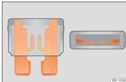
**Fig. 57** Image of a blown fuse.
