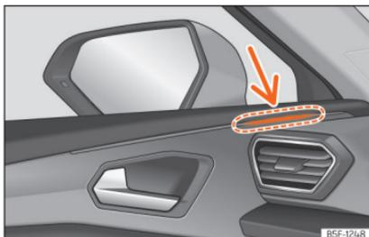
**Fig. 188** Control lamp of the lane departure warning.
