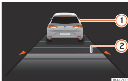
**Fig. 180** On the instrument panel display: ACC active.
