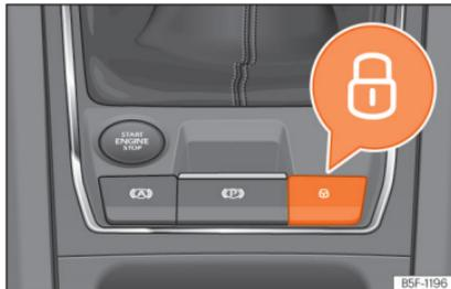
**Fig. 86** In the centre console: central locking switch
