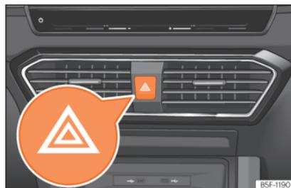
**Fig. 103** Dash panel: hazard warning lights switch
