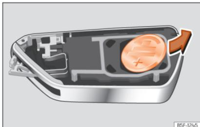
**Fig. 84** Vehicle key: removing the battery.
