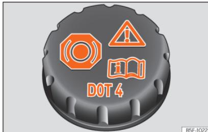
**Fig. 228** Engine compartment: brake fluid reservoir cap.
