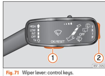
**Fig. 71** Wiper lever: control keys.
