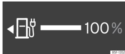
**Fig. 66** Digital instrument panel: battery level indicator.
