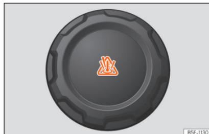
**Fig. 227** Engine compartment: coolant expansion tank cap.
