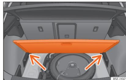
**Fig. 130** Variable luggage compartment floor: inclined position.
