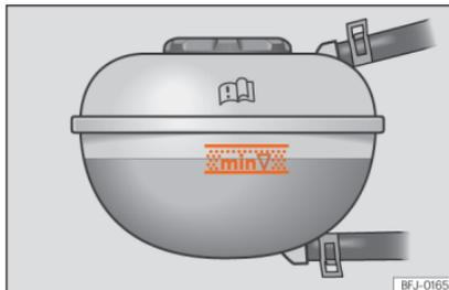
**Fig. 226** In the engine compartment: marking on coolant expansion tank.
