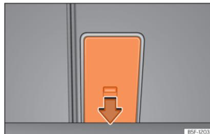
**Fig. 137** In the luggage compartment: opening the trapdoor.
