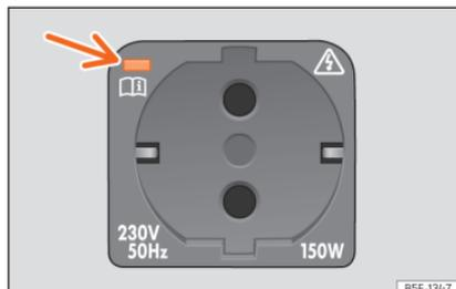
**Fig. 148** In the luggage compartment: 230 volt power socket.
