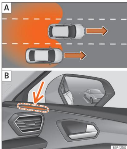
**Fig. 191** Schematic representation: **A** Situation of an overtaking in the centre lane and then moving into the right-hand lane. **B** Indication of the lane departure warning in the control lamp on the right side.
