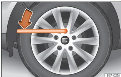
**Fig. 43** Wheel change: loosen the wheel nuts.
