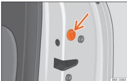
**Fig. 90** Locking the door manually.
