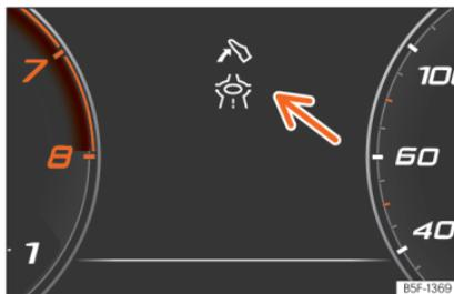
**Fig. 64** Eco-efficient driving assistance indication (schematic representation).
