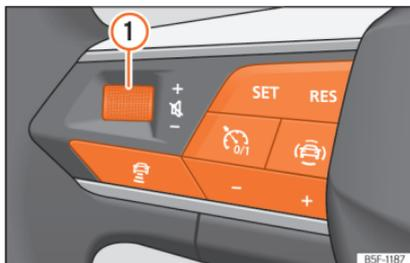
**Fig. 78** Controls on the steering wheel.
