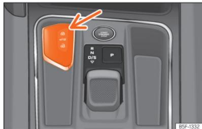
Fig. 81 Centre console: vehicle key socket.
