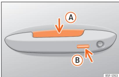
**Fig. 88** Door handle: sensor surfaces
