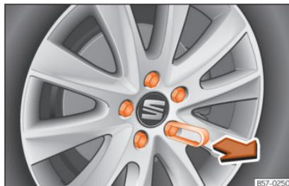
**Fig. 41** Wheel: wheel nuts with caps.
