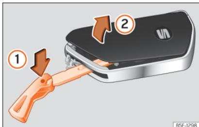
**Fig. 83** Vehicle key: opening the battery compartment cover.
