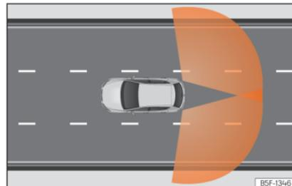
**Fig. 171** Sensor detection zones
