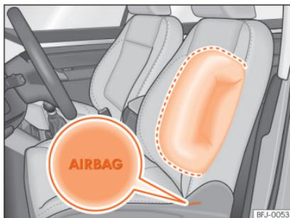
**Fig. 26** Side airbag in driver's seat.
