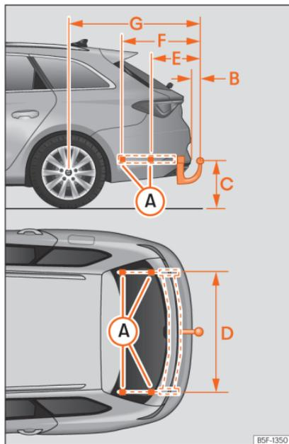
**Fig. 207** Limits and attachment points for retrofitting a towing bracket.
