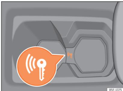
**Fig. 162** In the centre console: emergency start.
