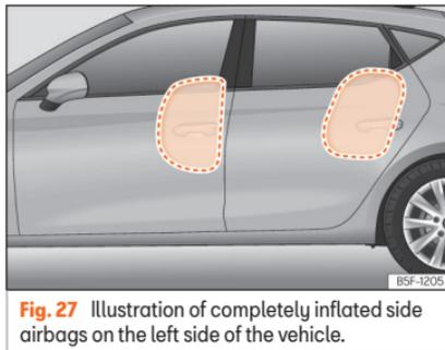
**Fig. 27** Illustration of completely inflated side airbags on the left side of the vehicle.
