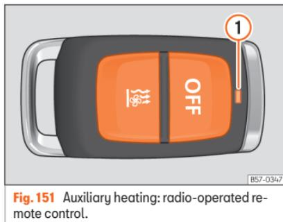
**Fig. 151** Auxiliary heating: radio-operated remote control.
