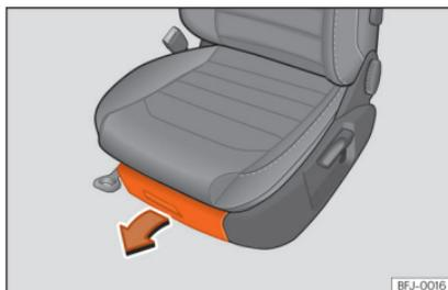
**Fig. 145** Drawer under the front seat
