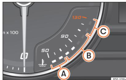
Fig. 69 Analogue instrument panel: engine coolant temperature indicator.
