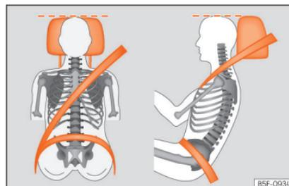
**Fig. 8** Correct belt web and headrest positions
