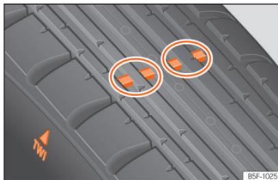
Fig. 234 Tyre profile: tread wear indicators.
