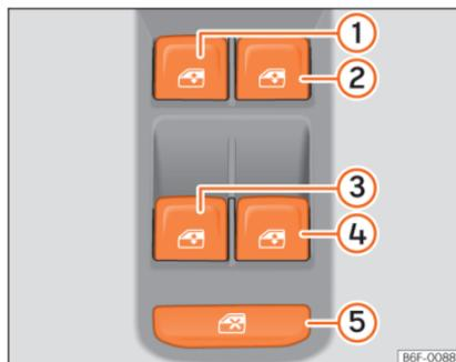
**Fig. 98** Detail of the driver's door: window controls.
