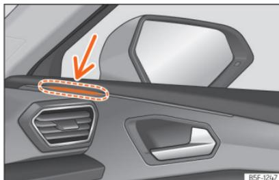
**Fig. 189** Control lamp of the lane departure warning.
