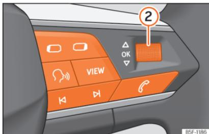
**Fig. 79** Controls on the steering wheel.
