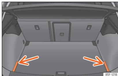
**Fig. 123** In the luggage compartment: covers for storing the rear shelf.
