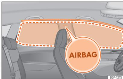
**Fig. 28** Location of head-protection airbags.
