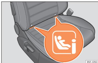
**Fig. 33** Front passenger seat: ISOFIX/i-Size securing rings.
