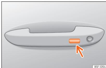
**Fig. 100** Door handle: sensor surface.
