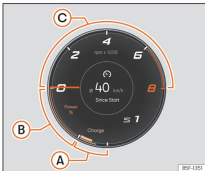
**Fig. 65** Digital instrument panel: Power meter
