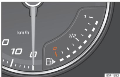
Fig. 67 Analogue instrument panel: fuel gauge
