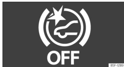
**Fig. 178** On the instrument panel display: Front Assist deactivated indication.
