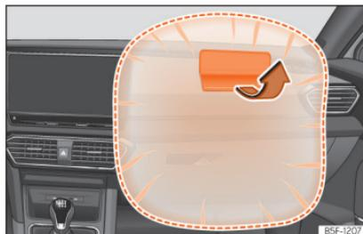
**Fig. 19** Front passenger airbag located in dash panel.
