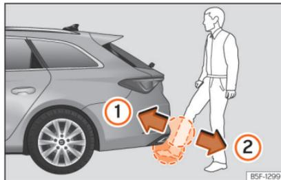
**Fig. 95** Rear lid with sensor-controlled opening (Easy Open).
