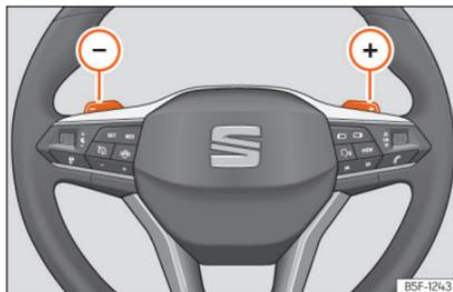
**Fig. 166** Steering wheel: automatic transmission levers
