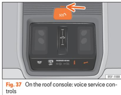
**Fig. 37** On the roof console: voice service controls
