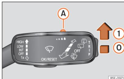
**Fig. 107** Wiper lever: adjust the rain sensor **A**
