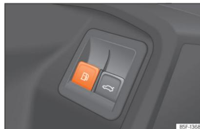
**Fig. 217** Driver's door: tank flap release.
