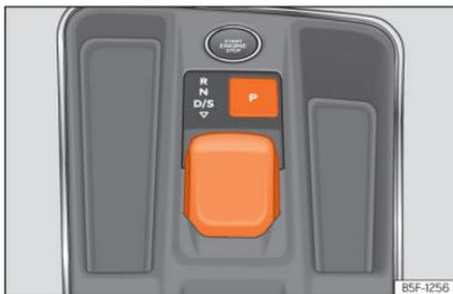
**Fig. 165** In the centre console: selector lever.
