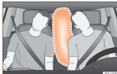
**Fig. 25** Fully inflated central airbag (deployment zone).
