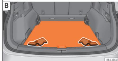
**Fig. 121** In the luggage compartment: adjust the height of the variable luggage compartment floor.
