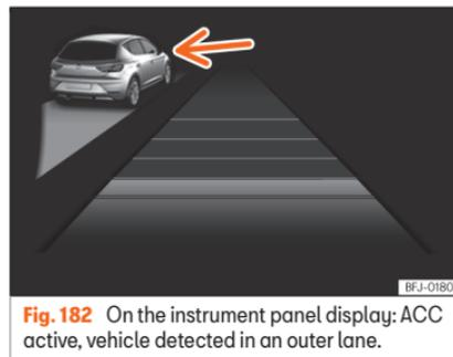
**Fig. 182** On the instrument panel display: ACC active, vehicle detected in an outer lane.
