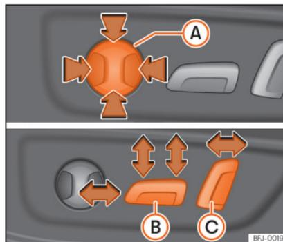
Fig. 100 Driver's seat: electric seat settings.
