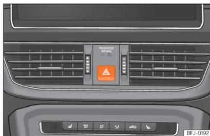
**Fig. 92** Dash panel: hazard warning lights switch
