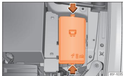
**Fig. 51** In the engine compartment: fuse box cover.
