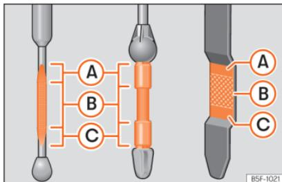
**Fig. 223** Engine oil dipstick.
