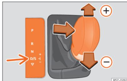
**Fig. 163** Lever in the Tiptronic position
