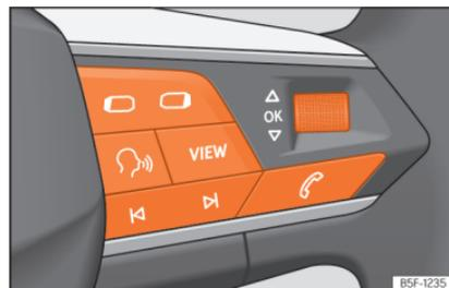
**Fig. 59** Right side of the multifunction steering wheel: buttons to the menus and information displays on the instrument panel.
