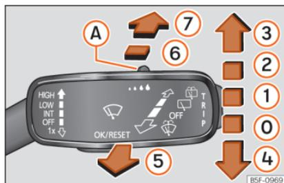
**Fig. 94** Operating the windscreen wiper and rear wiper.
