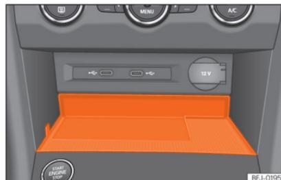
**Fig. 155** In the centre console: pad for the mobile phone connection.
