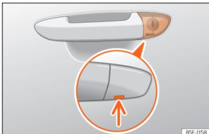
**Fig. 76** Driver door handle: Concealed lock cylinder.
