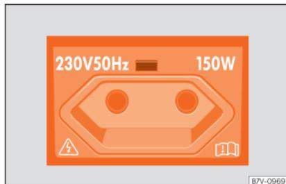
**Fig. 142** On the left side of the luggage compartment: 230 volt power socket.
