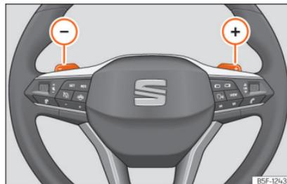
**Fig. 164** Steering wheel: automatic transmission levers
