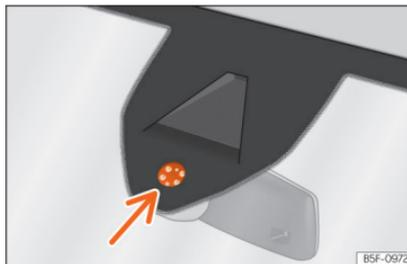
**Fig. 148** Windscreen humidity and temperature sensor.
