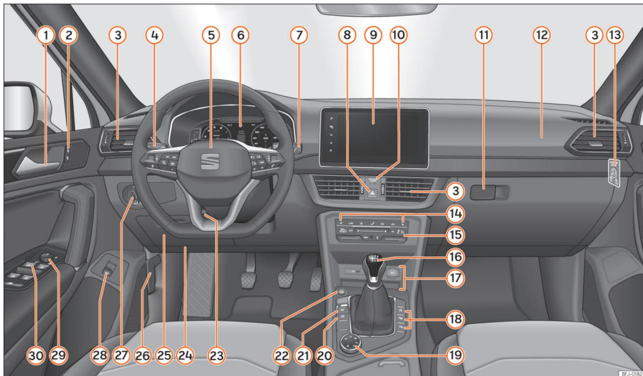
**Fig. 53** Instruments and controls.
