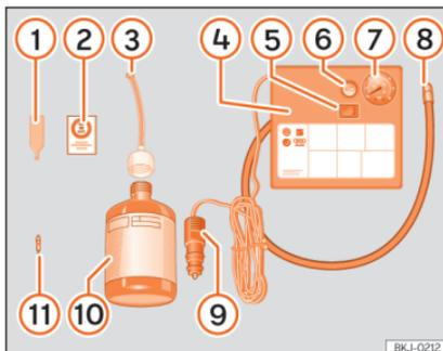
**Fig. 32** Standard representation: anti-puncture kit contents.
