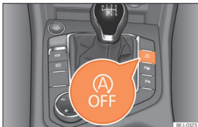
**Fig. 160** Centre console: Start-stop system button.
