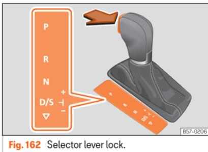
Fig. 162 Selector lever lock.
