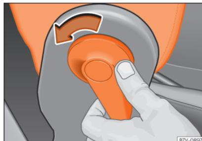
**Fig. 110** Unlocking the folding backrest of the front passenger seat
