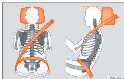
**Fig. 4** Correct belt web and headrest positions
