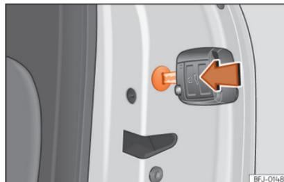
**Fig. 78** Locking the door manually.
