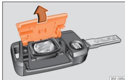
**Fig.70** Vehicle key: opening the battery compartment cover.
