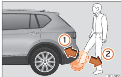
**Fig. 83** Rear lid with sensor-controlled opening [Easy Open].
