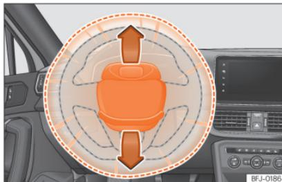
**Fig. 15** Driver airbag located in steering wheel.
