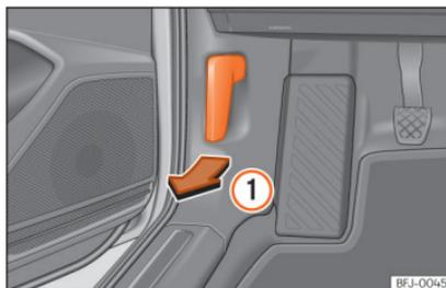
**Fig. 220** Release lever in the driver's footwell area.
