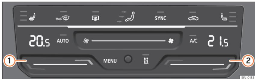
**Fig. 143** In the centre console: Climatronic controls.
