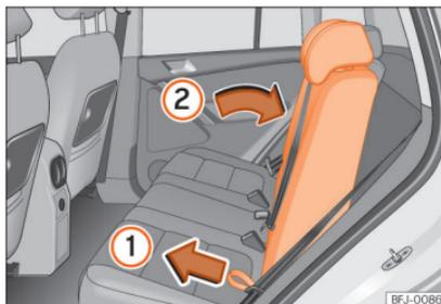
**Fig.102** Rear seat backrest adjustment.
