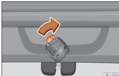
**Fig. 84** Detail of the luggage compartment: emergency unlocking
