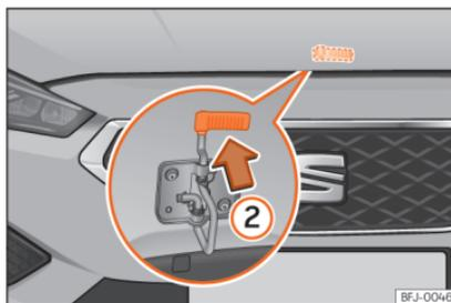
**Fig. 221** Cam under the bonnet
