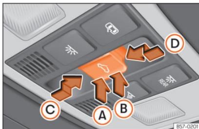
**Fig. 86** On the interior roof lining: sunroof button.
