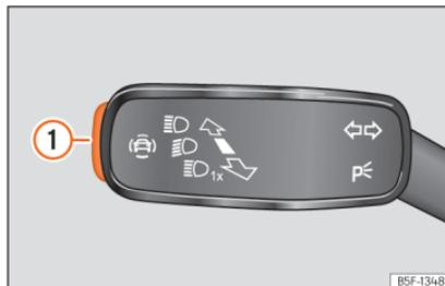
**Fig. 60** On the turn signal and main beam lever: button for driver assistance systems (depending on versions).
