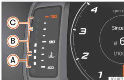
**Fig. 58** Digital instrument panel: engine coolant temperature indicator.
