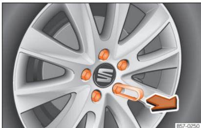
**Fig. 33** Wheel: wheel nuts with caps.
