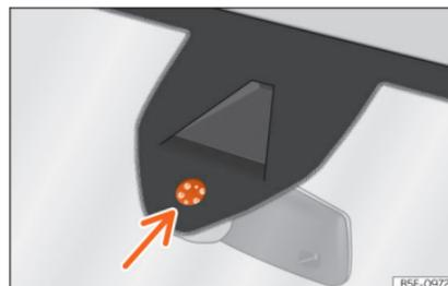
**Fig. 96** Rain sensor sensitive surface
