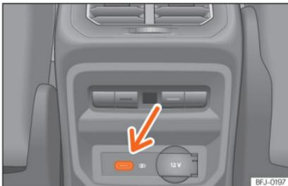
**Fig. 157** Rear part of the centre console: USB connectors with power outlet function.
