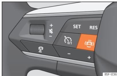
**Fig. 61** Left side of the multifunction steering wheel: button for driver assistance systems (depending on versions).
