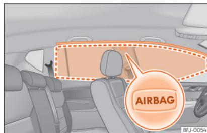
**Fig. 22** Location of head-protection airbags.
