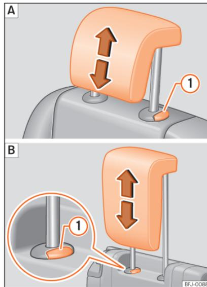
**Fig. 104** Adjusting the rear headrests: **A** Second row of seats, **B** third row of seats.
