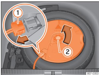
**Fig. 235** In the luggage compartment: remove the subwoofer.
