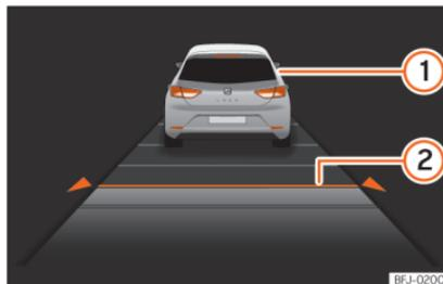
**Fig. 181** On the instrument panel display: ACC active.
