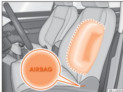
**Fig. 21** Side airbag in driver's seat.
