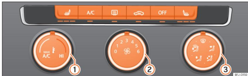
**Fig. 144** In the centre console: manual air conditioning controls.
