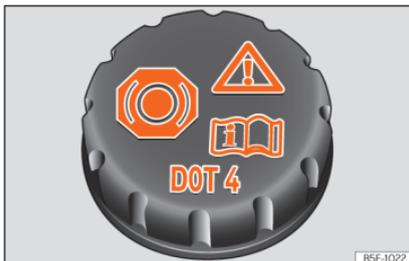
**Fig. 227** Engine compartment: brake fluid reservoir cap.
