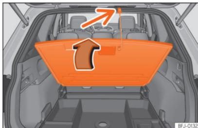
**Fig. 120** In the luggage compartment: lift the luggage compartment floor.
