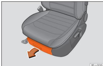
**Fig. 138** Drawer under the front seat
