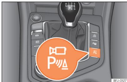
**Fig. 210** Centre console: button to manually activate/deactivate the peripheral vision system when combined with the park assist system.
