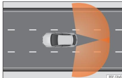
**Fig. 171** Sensor detection zones
