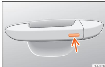
**Fig. 88** Door handle: sensor surface.
