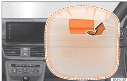
**Fig. 16** Front passenger airbag located in dash panel.
