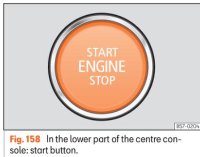
**Fig. 158** In the lower part of the centre console: start button.
