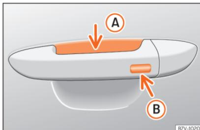
**Fig. 75** Door handle: sensor surfaces
