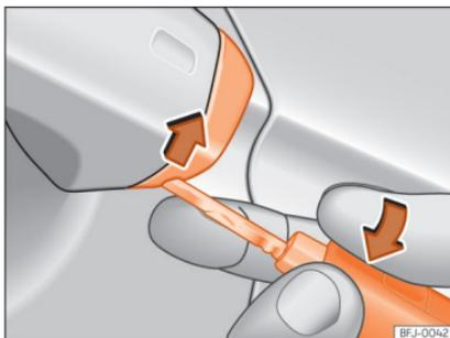
**Fig. 77** Driver door handle: lever the cover off
