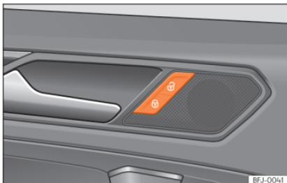
**Fig. 73** Driver's door: central locking switch.
