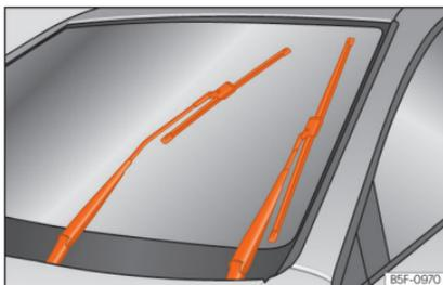
Fig. 40 Wipers in service position.
