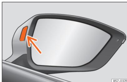
**Fig. 190** Control lamp of the lane departure warning.
