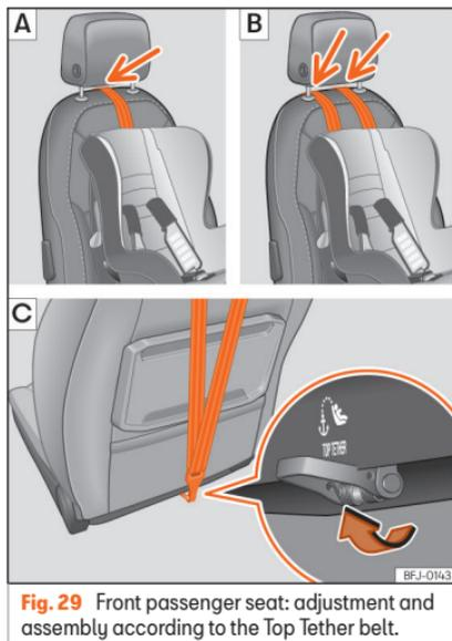
**Fig. 29** Front passenger seat: adjustment and assembly according to the Top Tether belt.
