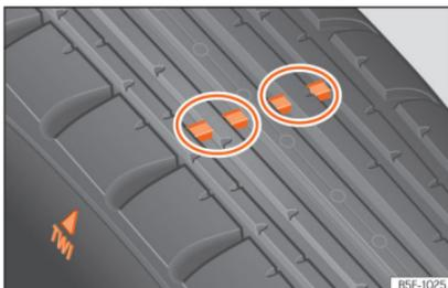
**Fig. 231** Tyre profile: tread wear indicators.
