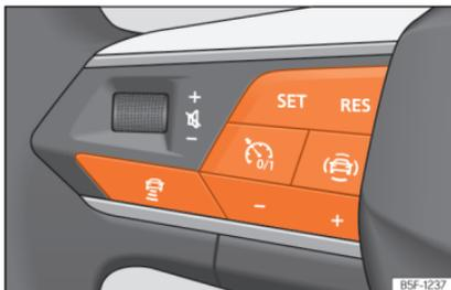
**Fig. 180** On the multifunction steering wheel: buttons to operate the ACC
