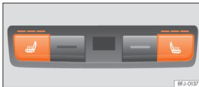
**Fig. 147** In the rear part of the centre console: rear seats heating switch.
