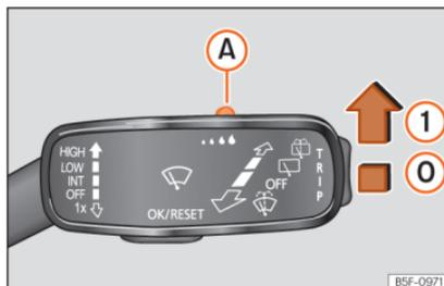
**Fig. 95** Wiper lever: adjust the rain sensor (A).
