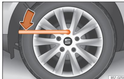
**Fig. 35** Wheel change: loosen the wheel nuts.
