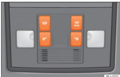
**Fig. 93** Detail of roof lining: front lighting of the passenger compartment.
