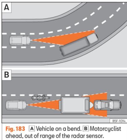
**Fig. 183** **A** Vehicle on a bend. **B** Motorcyclist ahead, out of range of the radar sensor.
