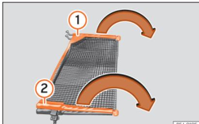
**Fig. 127** Deploying the net partition.
