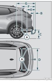
Fig. 180 Limits and attachment points for retrofitting a towing bracket.
