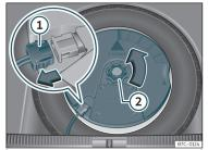
**Fig. 198** In the luggage compartment: remove the subwoofer.
