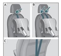
**Fig. 30** Front passenger seat: adjustment and assembly according to the Top Tether belt.
