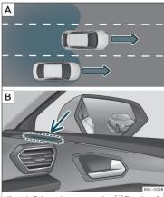
Fig. 163 Schematic representation: A Situation of an overtaking in the centre lane and then moving into the right-hand lane. B Indication of the lane departure warning in the control lamp on the right side.
