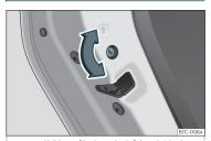
Fig. 76 Childproof lock on the left hand side door.
