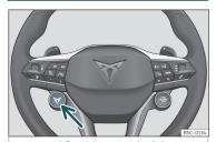
**Fig. 139** Multifunction steering wheel\*: button to change the driving profile.
